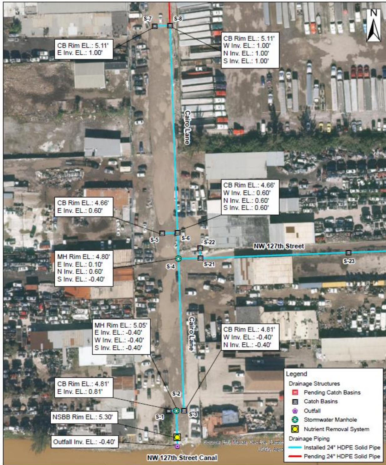
Figure 3. Drainage Infrastructure along Cairo Lane – Part 3
