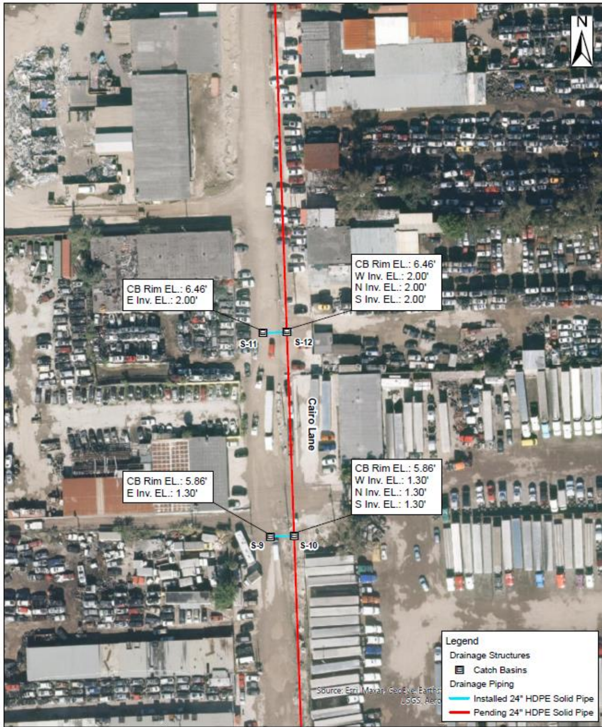
Figure 2. Drainage Infrastructure along Cairo Lane – Part 2
