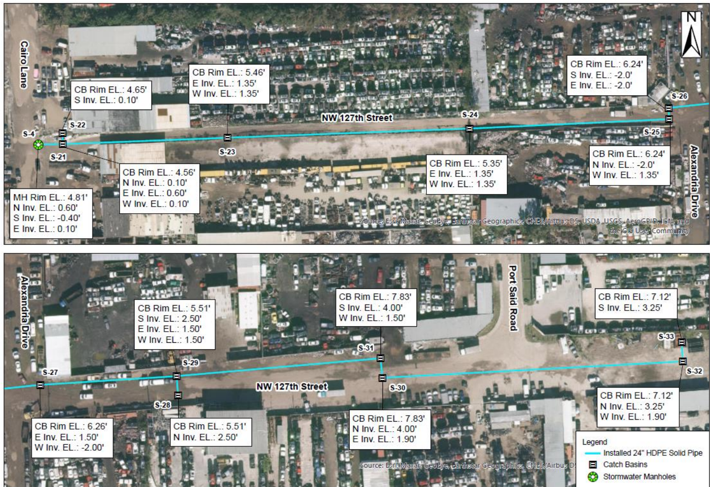
Figure 4. Drainage Infrastructure along NW 127 th Street
