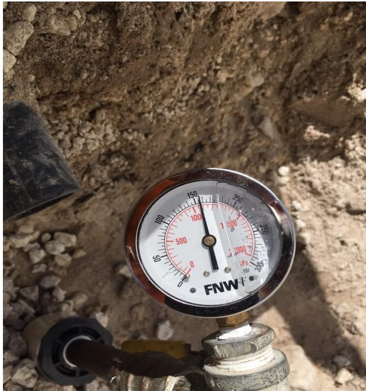
Pressure Gauge Reading 155 psi
