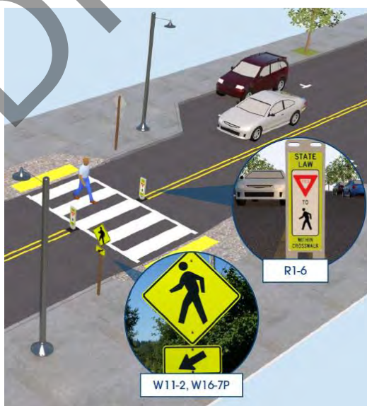
Figure 9-19: Example of Crosswalk Visibility Enhancement
