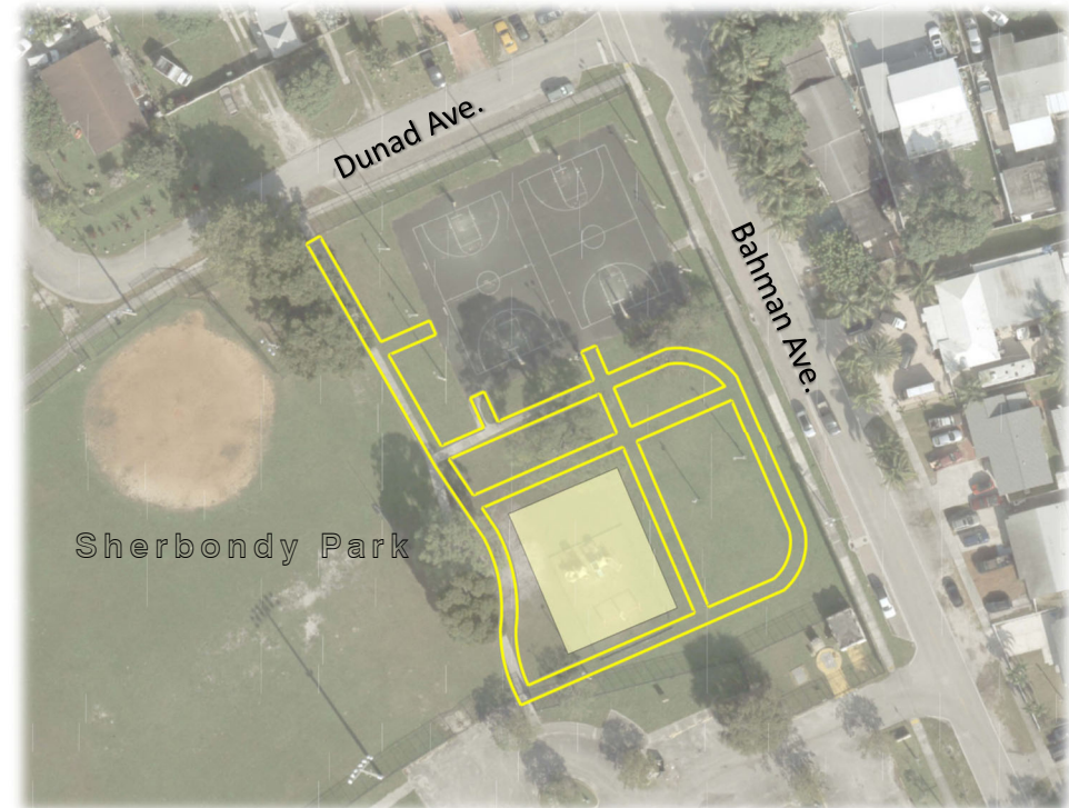
NEW 8ft.-wide Concrete Trails
